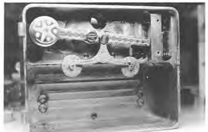
Figure 8b. The "block" in this photo is now lowered by the lever, thus unblocking the access hole.
