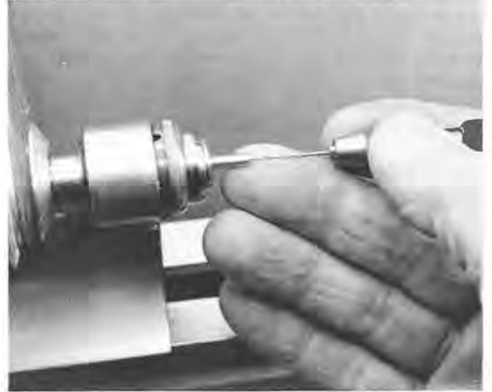
Figure 9. Drilling in a perfect center. Use your finger to support small bits.
