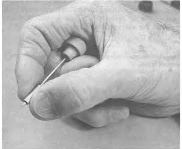
Figure 5. Hold the locator with thumb and finger.
