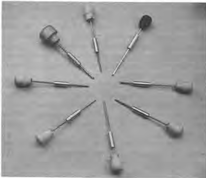
Figure 1. A group of center locating tools for lathe work.
