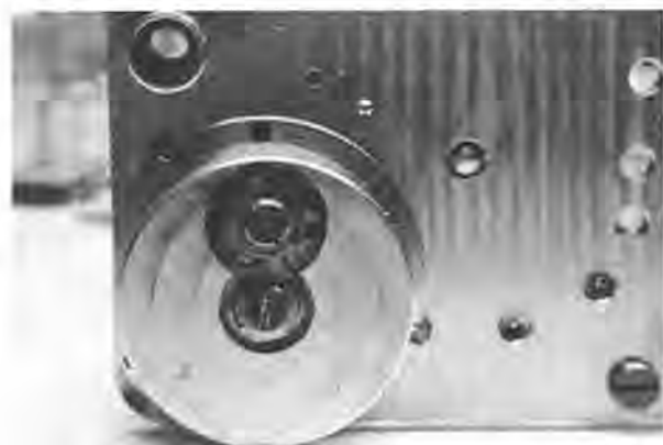
Figure 4. Conventional stopwork on the Yale #1.
