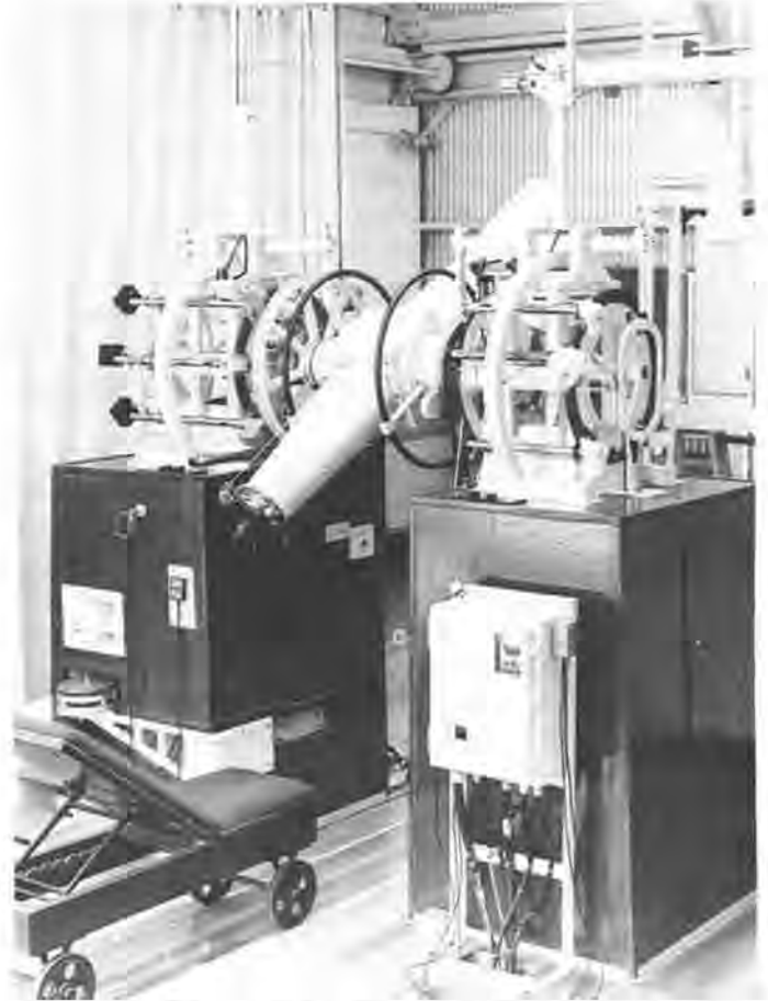
Figure 5. Six-inch Transit Circle. This telescope is so named because its lens is six inches in diameter, and because the east-west coordinate (the right ascension) of a star is measured by timing when it crosses, or "transits," the meridian due to the earth's rotation, while the north-south coordinate (the declination) is measured with a very finely divided circle. In both coordinates, precise measurements are made with respect to a system of wires placed in the focal plane of the eyepiece. The astronomer views these wires through the eyepiece and tracks the star with respect to them. These measurements, accurate to a few hundredths of a second of time, are immediately recorded by a computer for later analysis. After many observations, a catalog of star positions is produced, and in addition the positions of solar system objects are forwarded to the Nautical Almanac Office at the Observatory, where predictions are made of future positions (U.S. Naval Official Photograph).
