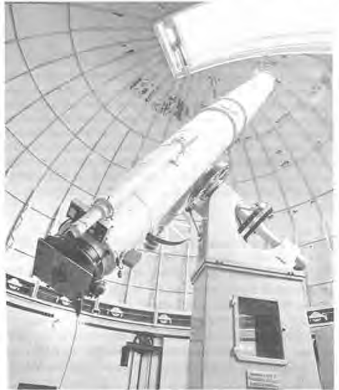
Figure 3. Clark's 26" Refracting Equatorial Mounted Telescope. The largest telescope at the Washington site of the Naval Observatory. It is primarily used for observing multiple star systems. The dome is 45 feet in diameter and can be rotated so that the shutter opening is exposed to the desired portion of the sky. Regular observation of the stars and other celestial bodies began November 20, 1873 (Official U.S. Navy Photograph).
