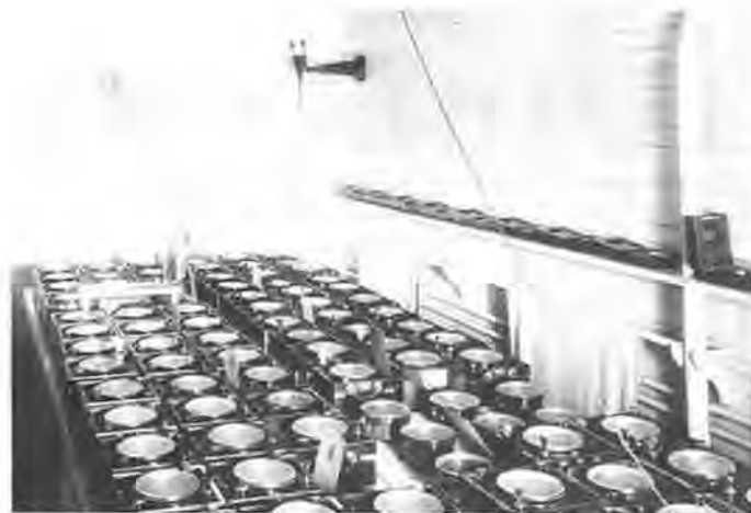
Figure 7. Naval Observatory Chronometer Trial Room prior to 1940. Generally, trials were held twice a year for a duration of six months. The trial number and temperature rate curve, showing the effect of temperature on the chronometer, was computed in five-minute increments from 50°F to 90°F by a special formula (U.S. Navy Official Photograph).
