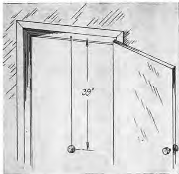
Figure 7. A good way to start experiments with simple pendulums is to hang a ball with string in a doorway. To begin, measure 39 inches from the point of suspension to the center of the weight.
