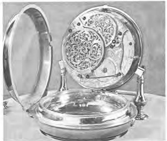
Figure 1. Views of the movement and dial of John Harrison's No. 4 timekeeper, constructed in 1759. On exhibition at the U.S. Naval Observatory, 1963, through loan by the British Admiralty. Forerunner of the modern marine chronometer, this timekeeper gained for Harrison an award of £20,000, offered by Parliament in 1714 for finding longitude at sea (U.S. Naval Observatory, Washington, D.C.).
