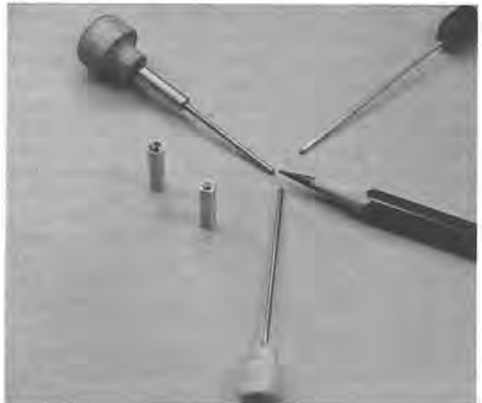
Figure 2. The drill has three edges with an included angle of 60 degrees.
