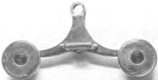
Figure 7. The "rollers" of the timelock mechanism, referred to in Mr. Stockwell's Patent (Figure 1) as the "rollers H & H," pivoting on a "split yoke G ."
