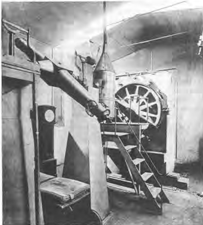
Figure 2. The 5.33-inch Transit Instrument, built by Ertel and Sons for $1,480, and 4-inch Mural Circle by Troughton and Simms, costing $3,550, mounted side by side at 23rd and E Street, N.W., site with a sidereal clock mounted against the south wall. The observer would note the time a star passed each cross-wire in the eyepiece. The Transit Instrument determined the star right ascension by the exact timing of the star's passage across the meridian. The Mural Circle could only determine declinations (U.S. Naval Observatory, Washington, D.C.).
