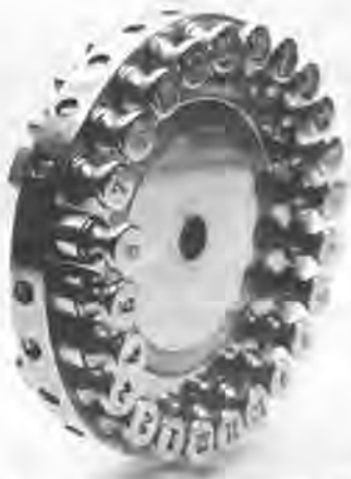
Figure 9. One of the two hour dials on this movement with 24 numbered friction pins upon which the rollers ride.
