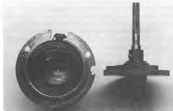
Figure 13. The barrel arbor, main wheel, and ratchet wheel assembly removed from the mainspring barrel.
