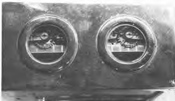
Figure 9. Top view of the case with the two glass apertures which allow viewing the balances.
