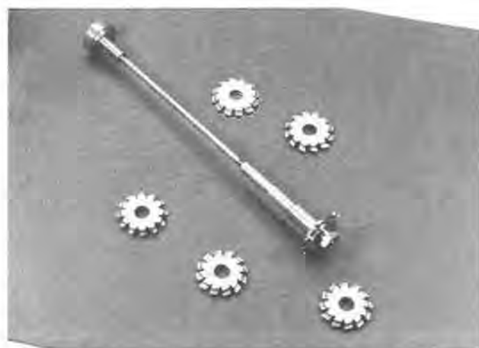
Figure 8. These gear cutters need a good strong arbor to be driven in a small lathe. The arbor shown is for the older Unimat machine.
