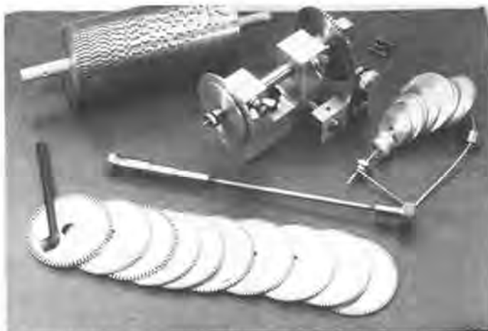
Figure 9. Index fixture, edge notched plates, cutter arbor, and other accessories for wheel making. These pieces were built for the older Unimat lathe, and adaptable to other small lathes.
