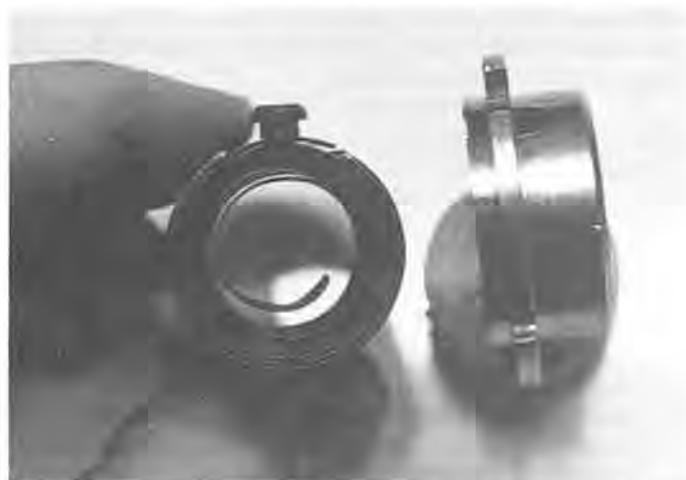
Figure 15. View of the mainspring with its large mushroom-shaped hook attached to the end of the mainspring and the attendant hook slot in the barrel wall.
