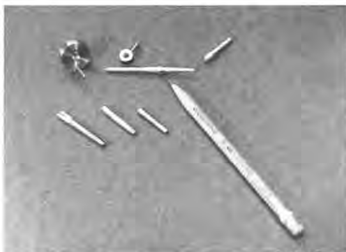
Figure 4. These pieces will turn most small lathes into highly precision machines, by the art of mandrel turning.
