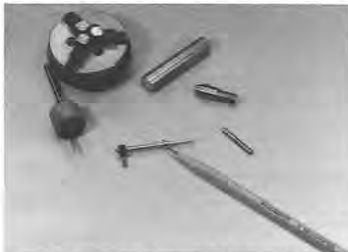
Figure 2. This small clock wheel hub is turned with very high precision in an older Unimat lathe with the aid of these simple fixtures.
