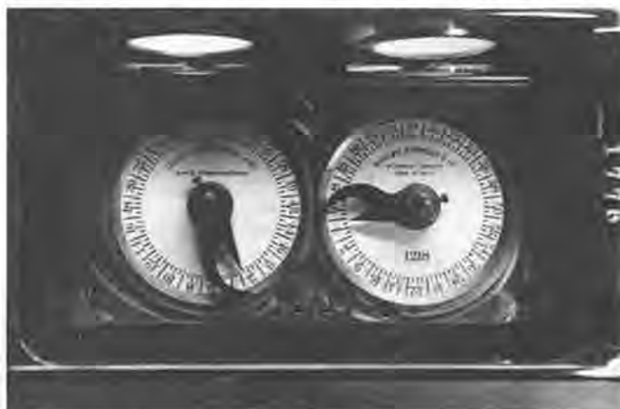
Figure 2. The Consolidated Timelock with its front cover removed. Note the glass apertures at the top of the case, which allow viewing of the two independent balance wheels.
