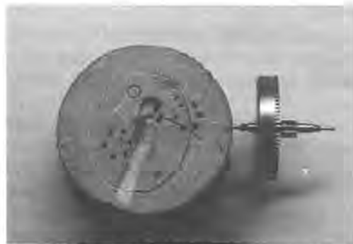
Figure 5. The contrate 5th wheel that transfers power from the train to the platform escapement.
