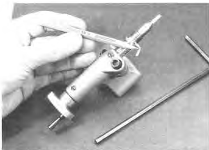
Figure 5. Rear view of the Unimat lathe tailstock. This modification permits use of small insertable tailstock fixtures.
