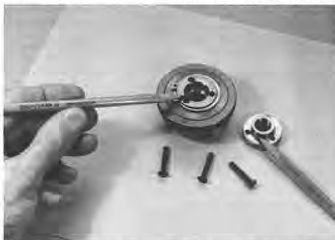
Figure 1. Run-out of a 3-jaw chuck is largely dependent on how the chuck back (L) fits onto the lathe spindle-hub (R).
