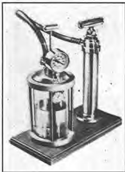
Figure 7. This waterproof testing device uses the vacuum principle in detecting leaky or faulty watch cases.
