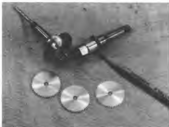
FIGURE 1. Wheel holding fixture and cutter arbor with finished wheels.
