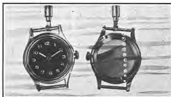
Figure 5. In the pressure test, air bubbles escaping from the watch case under water indicate the case has defects and is not water-protected.
