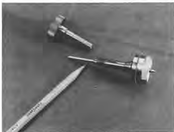
FIGURE 2. Wheel fixture with drawbar. Note that the wheel fixture extends through the lathe collet.
