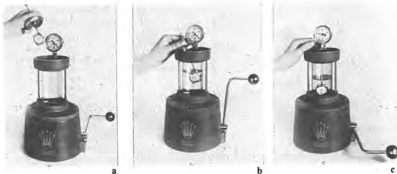
Figure 8. In another version of the vacuum test, the watch is placed in a water-filled jar, the water level of the jar is then lowered by means of a rubber-diaphragmed bottom and a partial vacuum created above the water level.
