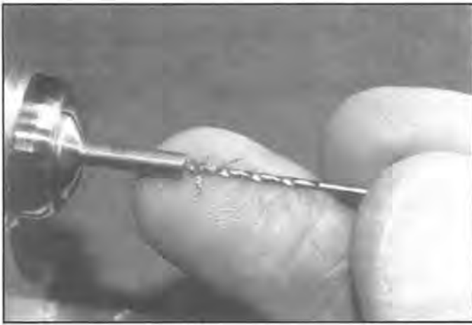
Figure 3. Drilling a brass rod to be made into a cup center. This will support and drive the wheel.
