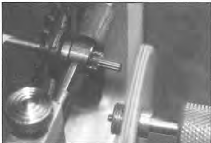
Figure 7. Use a high-speed grinder to kiss-off the bur left by the broken pivot.
