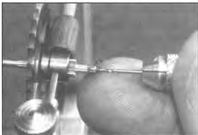
Figure 8. Locate center, and drill about five diameters deep. This bit is 0.0292" diameter. Support it on a finger tip.
