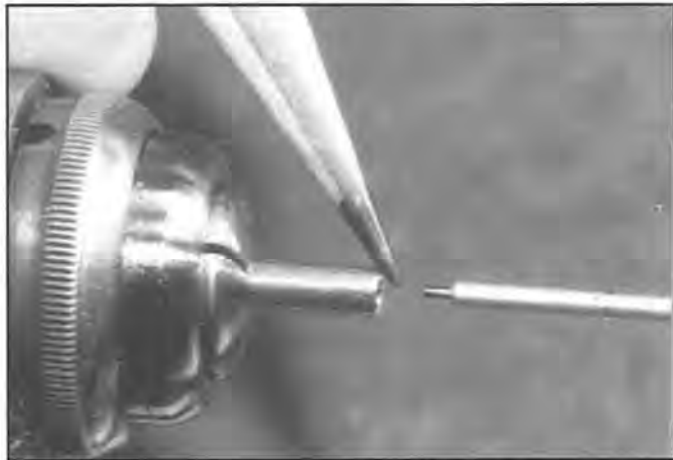
Figure 4. This pivot slips loosely into the drilled hole. The arbor shoulder will rest in the cup center.
