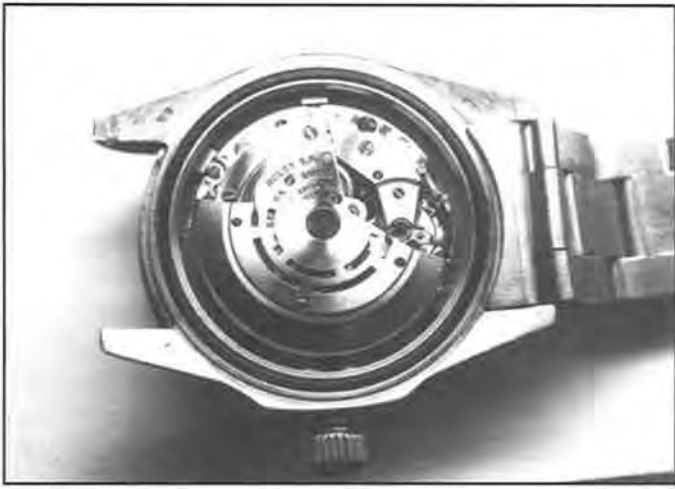
Figure 2. An O-ring case back gasket which rests in a channel or groove. The absence of a channel indicates a flat gasket needs to be used. The presence of a channel seat suggests an O-ring should be used.
