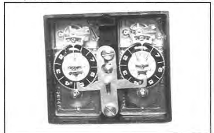
Figure 8. Argentinian Rench mini-timelock very similar to the LaGard version.
