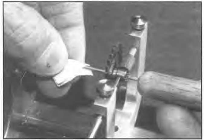
Figure 5. The wheel is supported by a bearing journaled on the pinion, held by a steady rest. Masking tape is used as a drive coupling.
