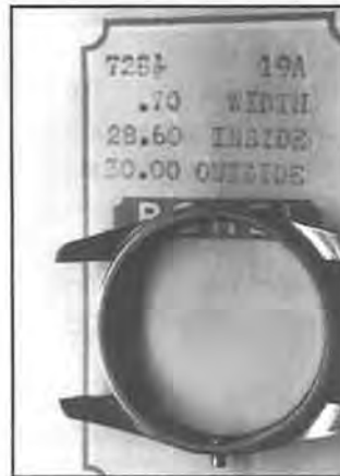
Figure 7. The selected replacement flat gasket in place in the case frame gasket seat.
