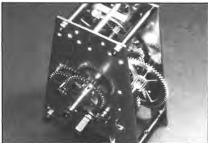
Figure 1. A broken pivot on the pinion-end of the escape wheel of this little movement is seemingly a very difficult job.
