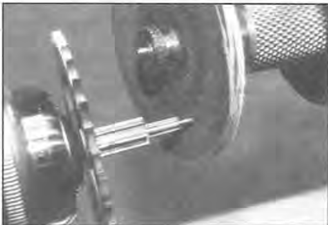
Figure 11. Grind the tip to length where run-out is a problem. Do this in a steady rest.
