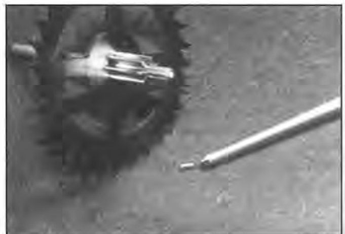
Figure 2. Repivoting this one appears to be extremely difficult: too much overhang to be collet-held.
