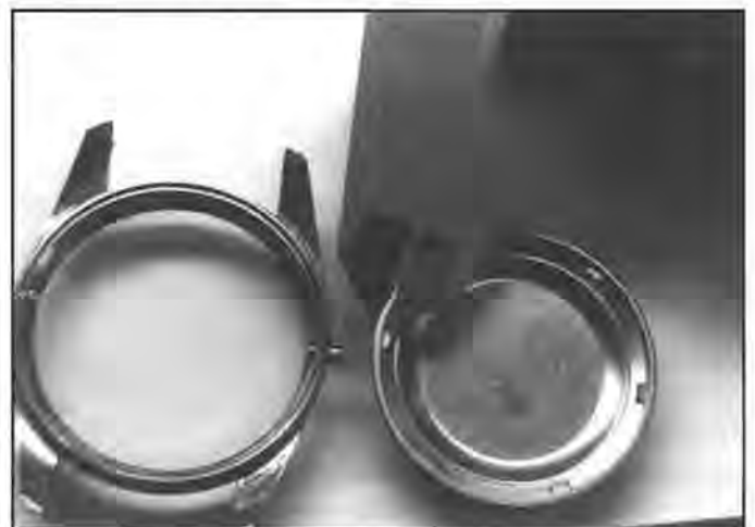
Figure 1. Measuring the width of the case back gasket seat for a flat gasket. Note the lack of a groove or channel in which the gasket could seat.
