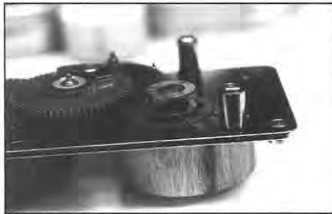
Figure 2. The unique planetary gear incorporated into the fifth wheel and controlled by the dial, gives a rapid release of unlock power to this movement.
