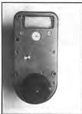
Figure 5. Rear view of the movement. Note the mainspring barrel which houses the mainspring that powers the release lever.
