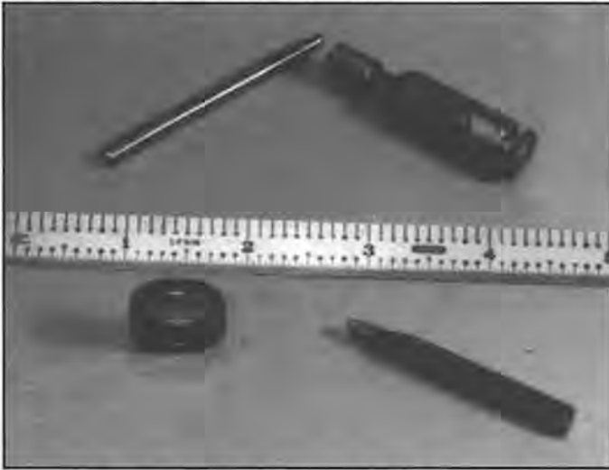
Figure 8. The Hammel Riglander Tool Post as supplied with the 3-deck tool slide.
