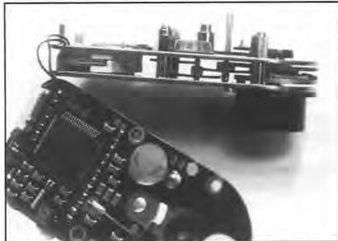
Figure 9. Side view of the movement with the circuit board removed.
