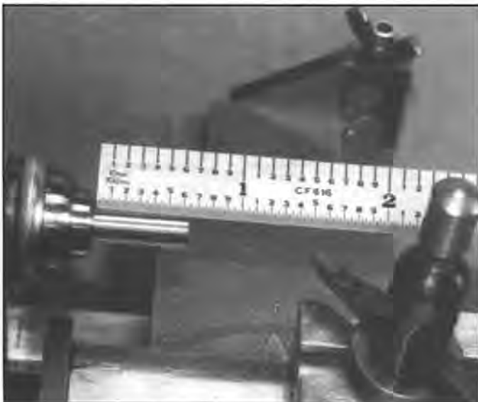
Figure 9. The workers eye-view of the Tool Post and Bit.
