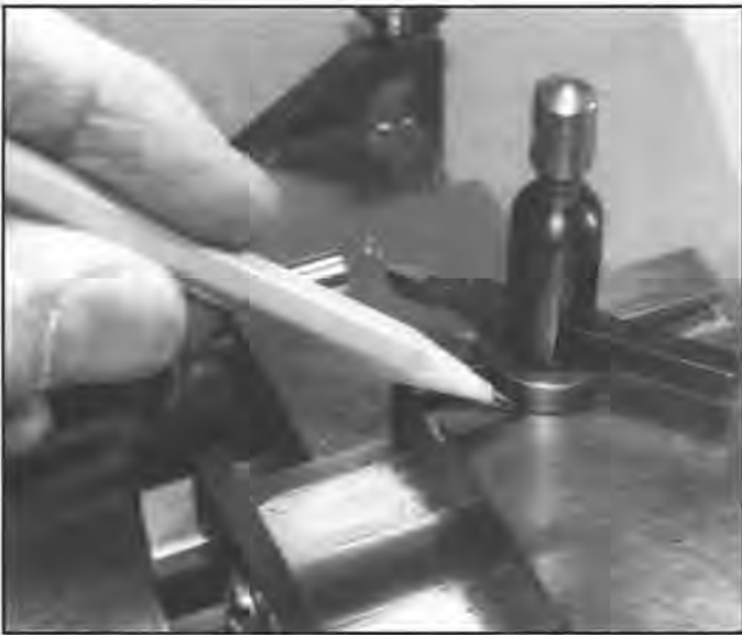
Figure 7. Thickness of this swashed spacer adapts the tool slide rest to your lathe spindle height.
