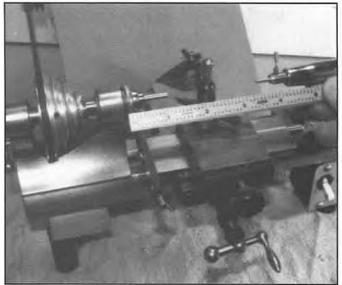
Figure 4. Work length overhang is a never ending problem. This piece is just over 1/2" long.
