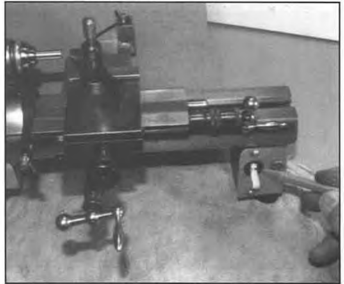
Figure 5. A convenient switch and constant speed motor improves productivity.
