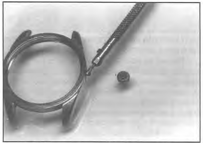
Figure 5. Lubricating the outside of the case tube prior to replacing the O-ring crown onto its case tube.
