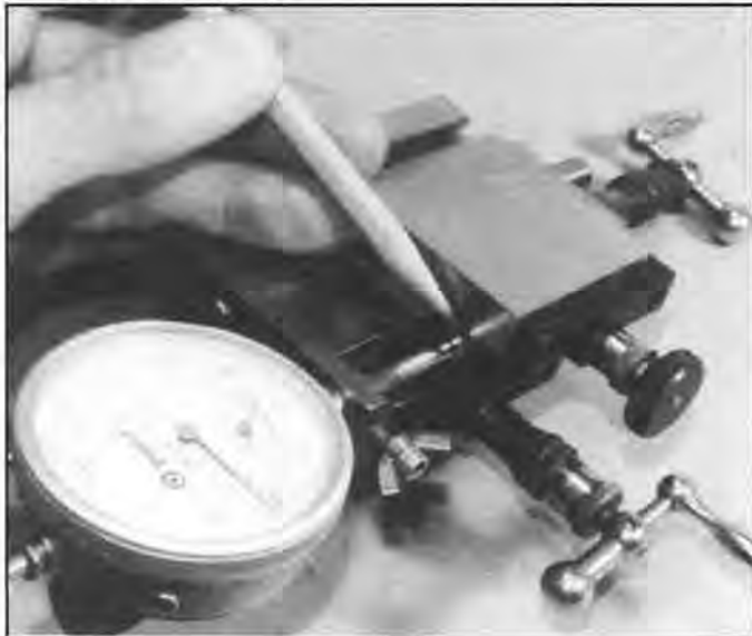
Figure 2. Tip of dial gauge to read longitude motion. Wing nut and bracket holds dial gauge in place.
