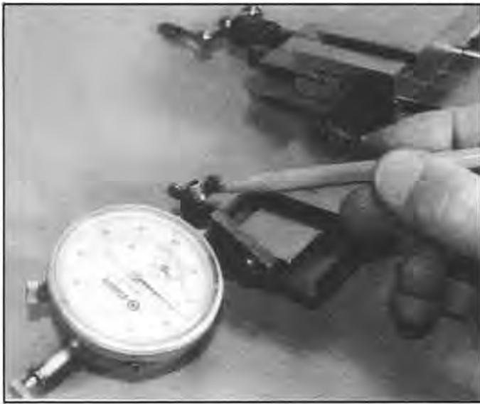
Figure 1. Cross-slide rear end showing lock nut and bracket for dial gauge.
