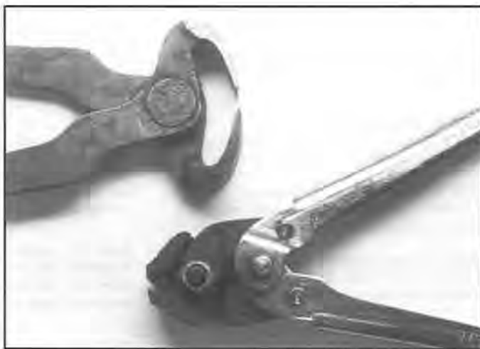
Figure 5. A pair of large nippers used to cut mesh watch bands to length (top) along with a pair of compound-leverage clippers designed specifically for this task.
