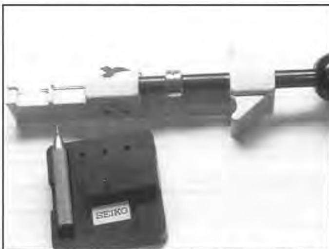
Figure 4. Two link pin removing tools, one from Citizen Watch Company (top) and one from Seiko.
