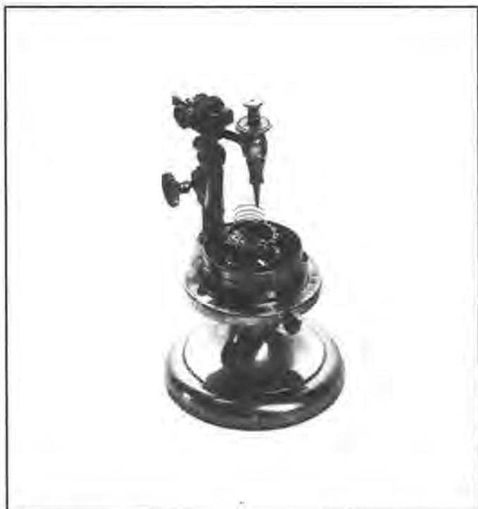
Figure 65. How a sample balance is suspended over a glass-enclosed master balance.
