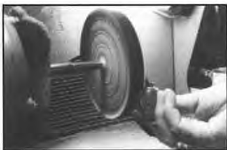
Figure 1. Bright finish on case on buff wheel with Fabulustre.
