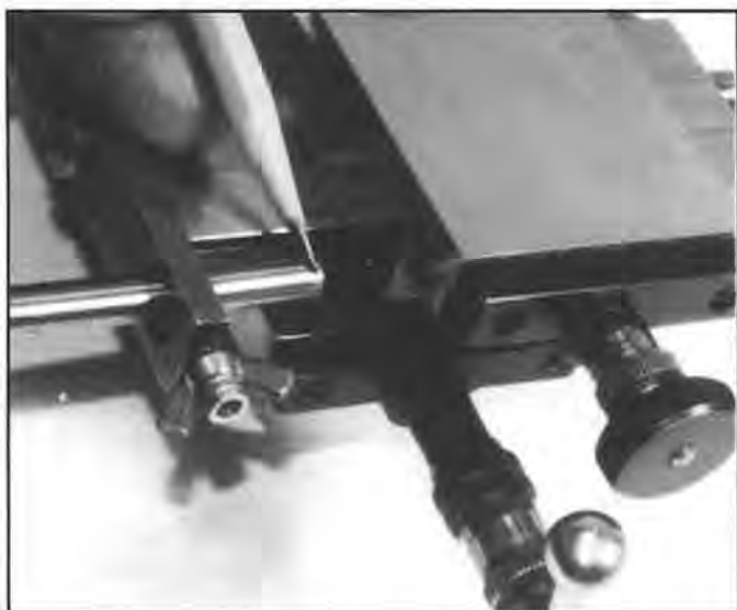
Figure 7. Safety stop to limit longitude slide range.
