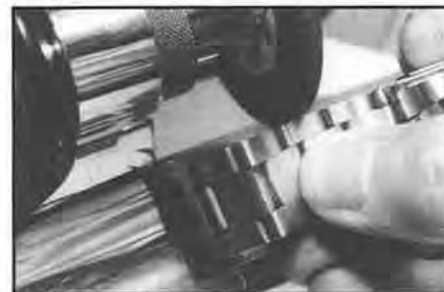
Figure 8. Side of link receiving a line finish.
