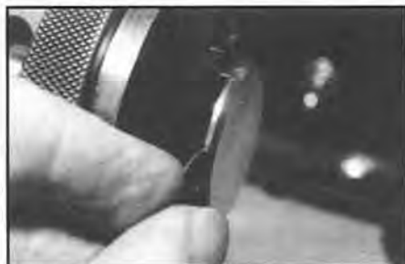
Figure 2. Round case back in three-jaw chuck, spinning to remove pits and rust with broken cut-off wheel.
