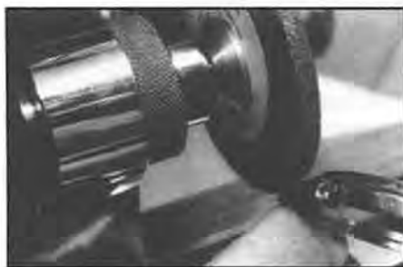
Figure 5. Mid-frame of case receiving a slight curved finish with a coarse Cratex wheel.
