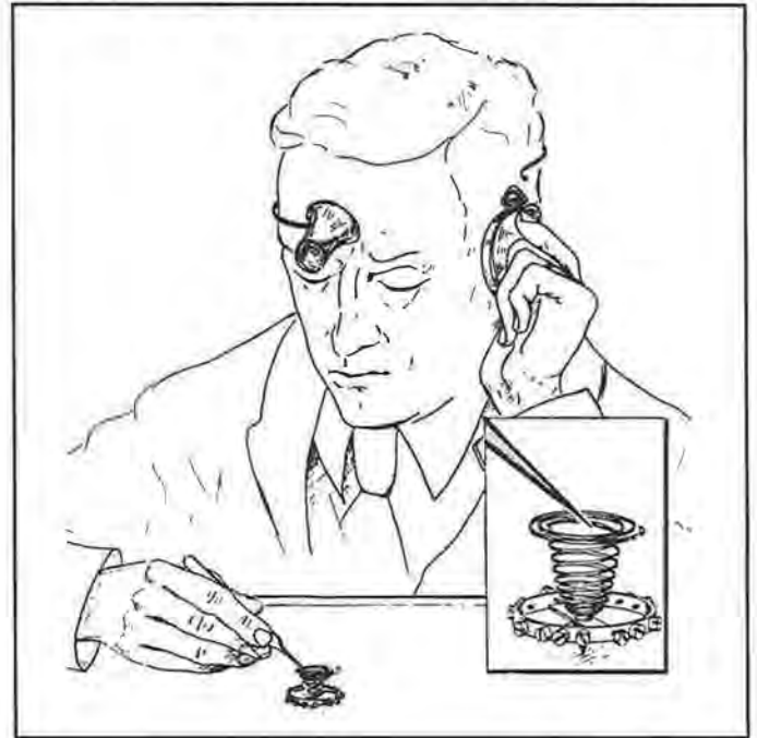
Figure 69. Another method is to suspend the balance and to observe the vibrations, timing them by the sound of a going watch held against the ear.
