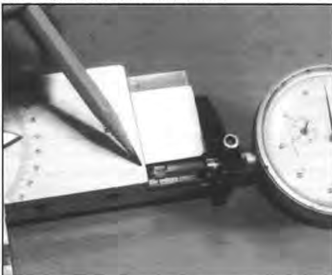
Figure 9. Dial gauge fit-up on the Hammel Riglander tool slide rest. This is the cross slide.
