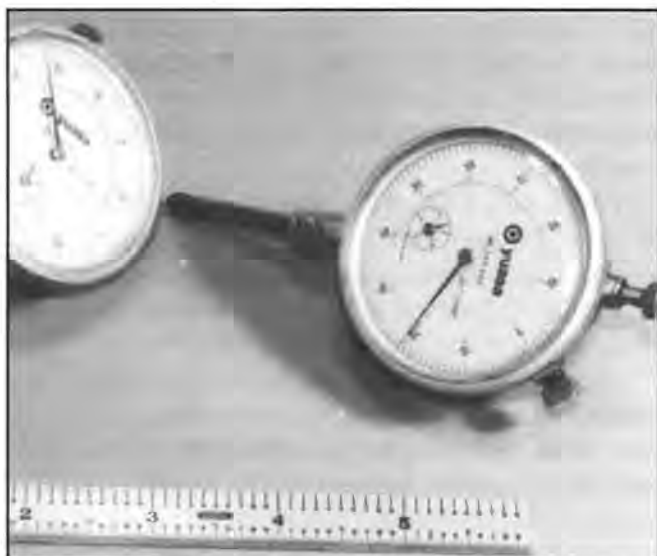
Figure 8. Dial gauges used with the modified tool slide rest. Divisions are 0.001" slide motion.
