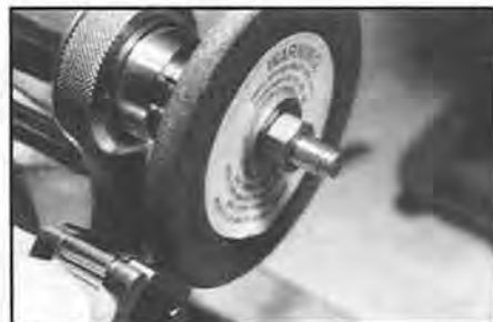
Figure 6. Watch band link receiving a straight-line finish with a medium-grit Cratex wheel.
