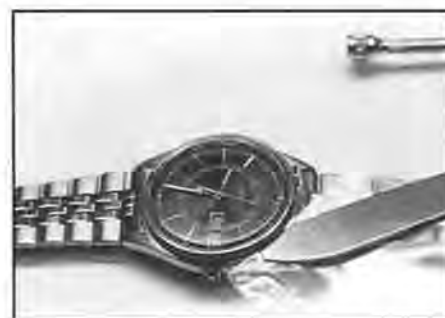
Figure 17. Removing decorative bezel ring using a folded piece of poly bag to protect the case finish. This bezel ring also provides protection for the upper portion of the armored or tension ring crystal. The crystal itself seats on the inside of the case frame as in Figure 16 using a stepped tension ring to hold the movement.
