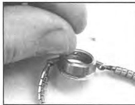
Figure 5. Round cylinder crystal: straight-sided crystal, hollow in the inside to give room for the watch hands, snaps into the straight-sided watch bezel.
