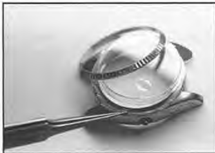
Figure 9. On many of these inexpensive watch cases, where a genuine replacement crystal is not available, pick a generic replacement crystal that fits snugly into the crystal bezel ring and then cement the bezel and crystal to the case frame by applying an epoxy around the case frame rim.
