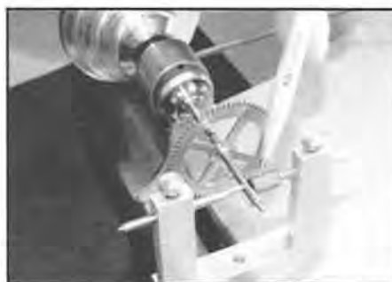
Figure 7. The steady rest setup is shown. This wooden dowel permits high-speed operation at zero clearance.
