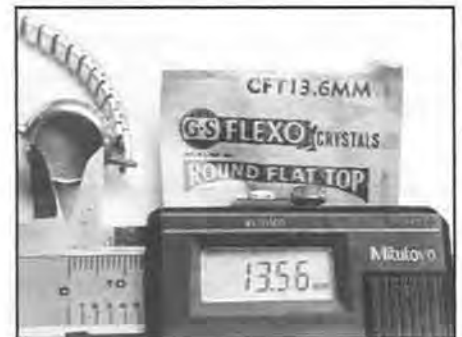
Figure 7a. Measure the inside of the bezel to get the needed size; in this case the crystal bezel is part of the case frame and takes a round cylinder crystal.
