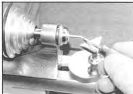
Figure 6. A cup center is cut in a piece of brass rod. This will support and drive our repivoting work.
