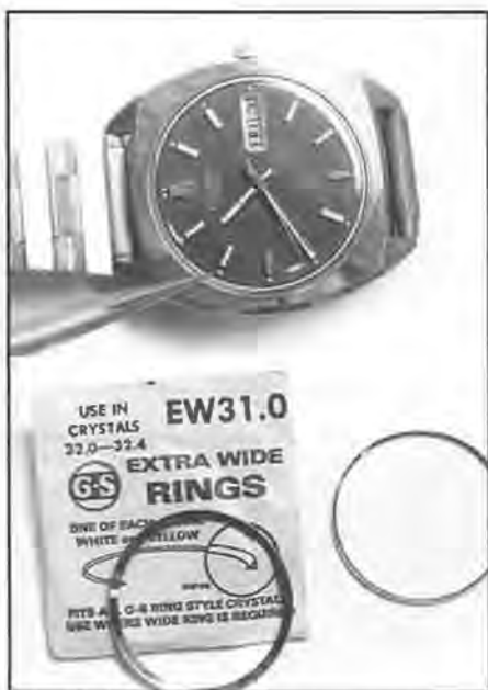
Figure 15. Cases with a wide gap between bezel and dial edge require a wide tension ring to keep the dialed movement in place.
