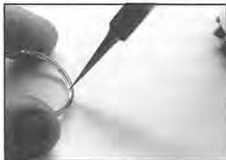
Figure 16a. A “stepped” tension ring is required to hold some movements in place.
