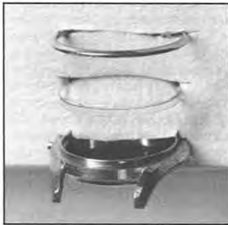
Figure 3. The round press-on crystal: the straight-sided crystal fits snugly over the raised rim on the case frame.
