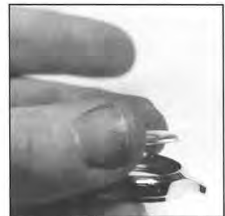
Figure 14. Bezels with angled or beveled walls require only the flexible type crystals.
