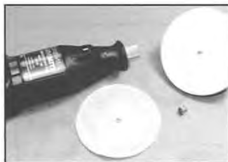
Figure 3. Modern abrasive paper on a soft-backed disc is driven in a battery-powered motor tool.
