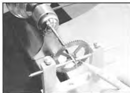
Figure 8. A smaller dowel is used if the arbor length is short.
