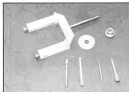
Figure 4. A steady rest is needed for repivoting work. It is not suitable for turning.
