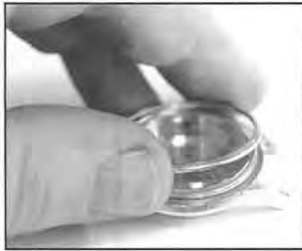
Figure 4a. The bezel ring then fits tightly around the outside of the crystal creating a sandwich in which the outer bezel ring holds the crystal firmly against the inner rim of the case frame.
