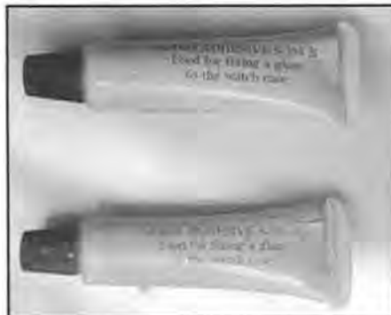
Figure 10. Seiko two-part crystal epoxy: a flexible, resilient epoxy for sealing loose crystal to case frames. Works especially well for filling in gaps created by a crystal that is too loose a fit in the case. Yet this epoxy can be easily removed by heating the case and crystal.
