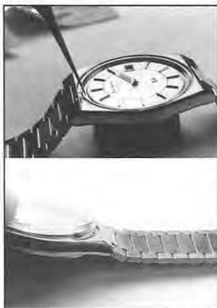
Figure 16b. In some thinner watch cases, the dialed movement sits above the crystal seat. This is done to give a deeper wall for the crystal to seat against. The stepped tension ring provides a wider pressure surface on its outer diameter and a recessed step to hold the movement in place.
