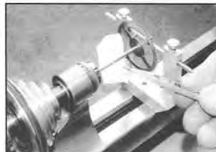
Figure 10. The coupling is a piece of paper masking tape.
