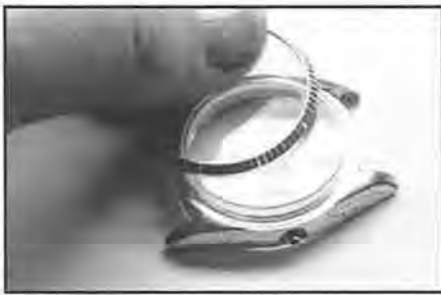
Figure 8. In very inexpensive watch cases, the crystal that fits snugly over the case frame rim has walls too thin for the outside bezel to fit firmly around the outside of the crystal and hold the crystal in place. Primarily because the crystal (with thicker walls) is not available as a replacement crystal.
