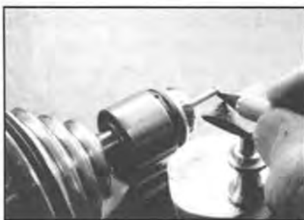
Figure 5. A cutoff tool is used in many types of lathe work. This one cuts mild steel and brass with ease.
