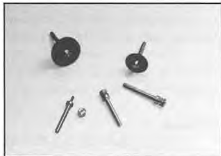
Figure 2. Thin rotary stones are used to cut very hard, prefinished pivot material.
