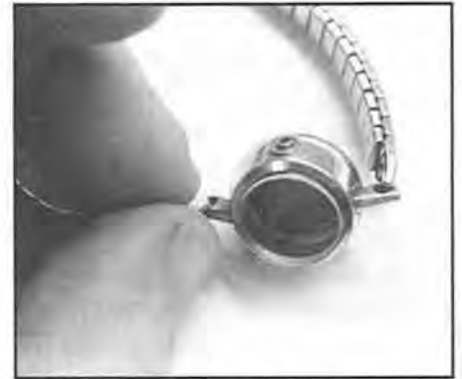
Figure 6. Sealed in place with crystal cement applied around the circumference of the bezel recess.
