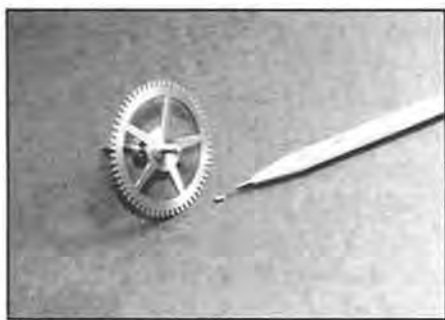
Figure 1. A broken pivot is shown. The following tools solve that problem quickly.
