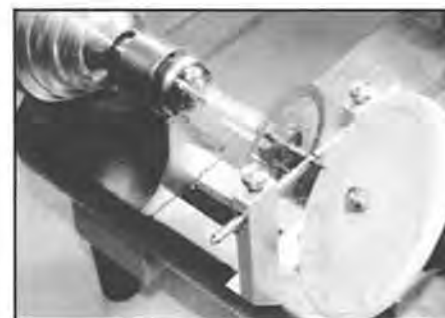
Figure 12. Grinding the conical tip on an inserted pivot.
