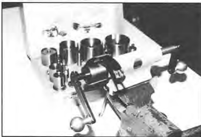
Figure 4. Bergeon spring winder.
