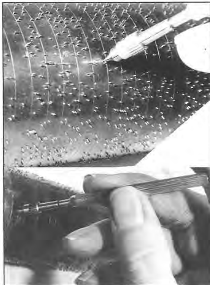
Figure 14.4. Pin straightening tool.
