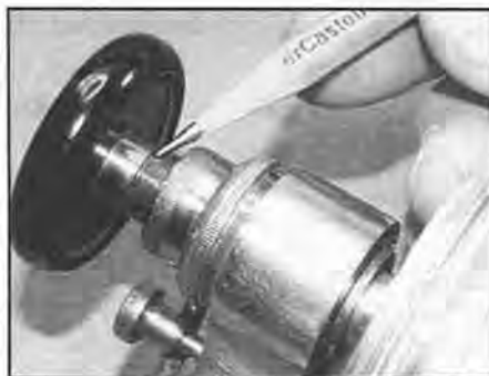
Figure 4. Joint line of lathe spindle and drawbar shoulder. A spacer is to be used here for collet adaptation.
