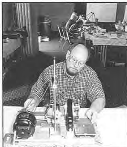
Truett Underhill cuts a watch wheel during the Phase IV Wheel Cutting course conducted in Charlotte, NC, February 14-17, 1997.
