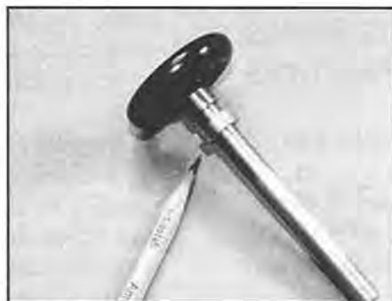
Figure 5. The spacer should have square ends and a snug fit onto the drawbar.
