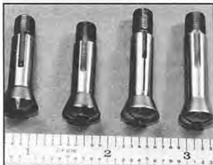
Figure 1. Relative size of typical 8-mm collets. These are: Peerless WW, English-made WW, genuine Moseley, Starrett made for Moseley.
