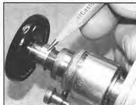
Figure 7. A Boley lathe with drawbar spacer for use with a longer collet.
