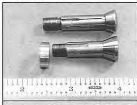
Figure 2. Genuine Moseley and an English-made WW collet. This drawbar spacer permits use of Moseley collet in a WW lathe.
