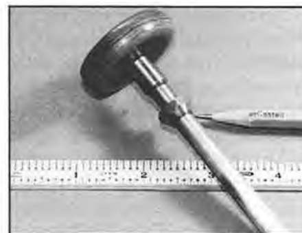
Figure 9. This Pennant lathe drawbar has a conical shoulder. The spacer ends are cut to fit that shape.
