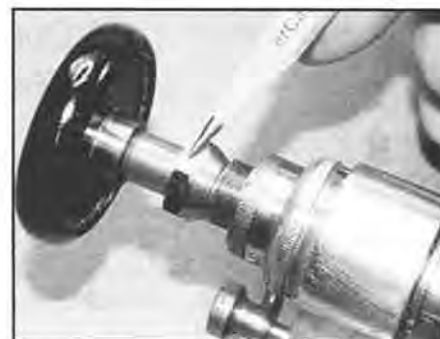
Figure 8. An alien drawbar may use a conical-end spacer to locate the drawbar in spindle center.
