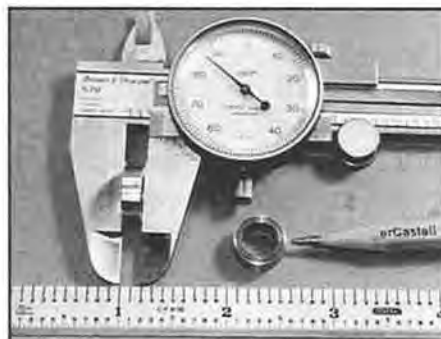
Figure 6. This spacer is 0.186" long. One or two lengths will solve most needs.
