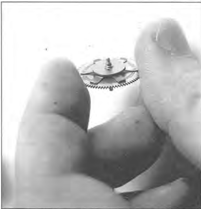
Figure 6. "Backwindable" third wheel, available in either the Style "S" or the Style "R".
