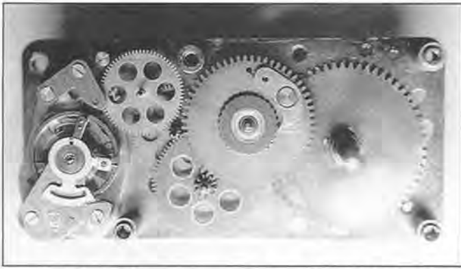
Figure 5. Style "S" movement with "non-backwindable" (non-resettable) third wheel clutch.
