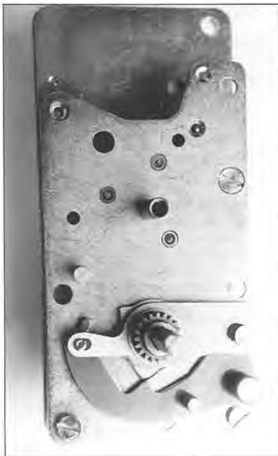
Figure 12. Note the snap-action cam on the winding arbor with a rounded lobe and a peaked lobe.
