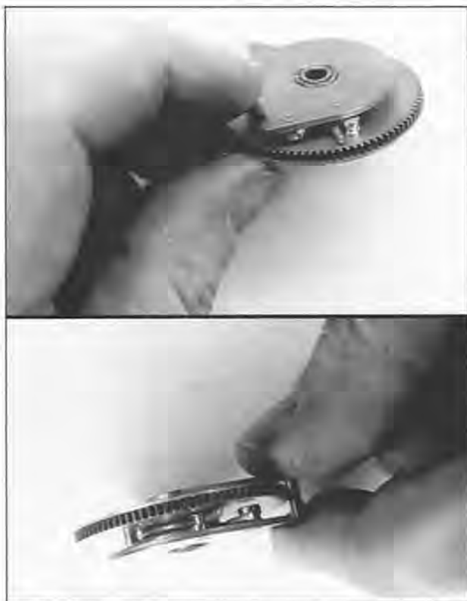
Figure 15. Indicator dial/gear wheel assembly positioned so that the stiff snap-action spring touches the heavy pin on the gear wheel in preparation for installing onto the movement.
