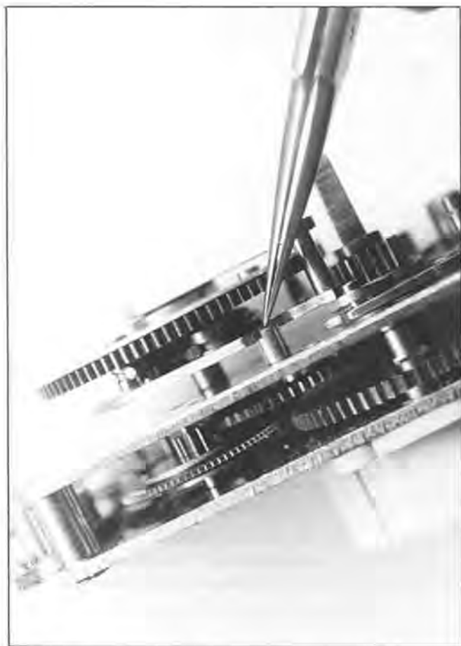
Figure 16B. Dial/gear wheel assembly inserted halfway onto the center post with the horn of the gear wheel hooked onto the top of the large pin (indicated by the tweezer point).
