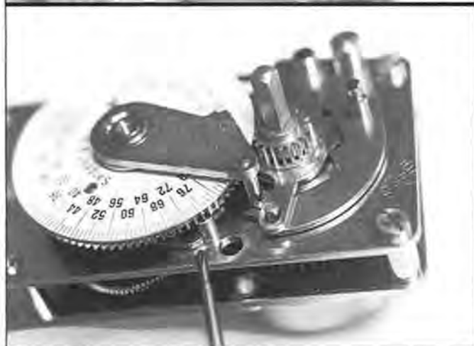
Figure 18. With the spring tension loaded onto the dial/gear wheel assembly, the unit is pressed fully onto the center post, meshing the gear wheel teeth with the winding pinion.
