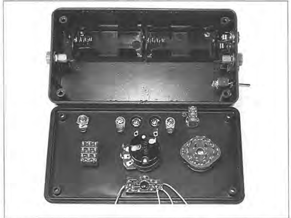
Figure 10. The majority of the components mounted and ready for wiring.
