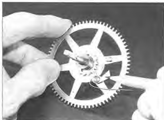
Figure 1. Failure of the click, its rivet, spring, or the ratchet can wreck the movement.
