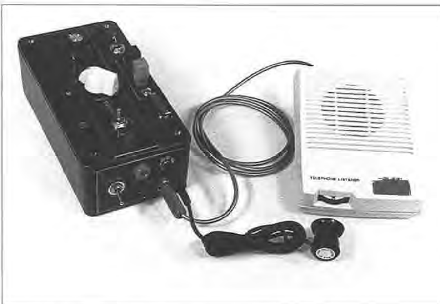
Figure 13. The completed analyzer shown with the Radio Shack Telephone Listening amplifier, its induction pick up coil, and an audio patch cable.
