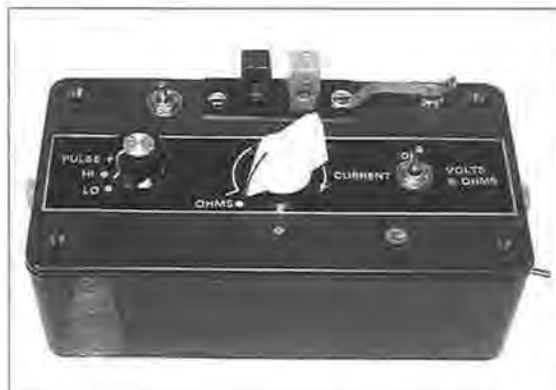
Figure 1. The 22-function quartz watch analyzer.
