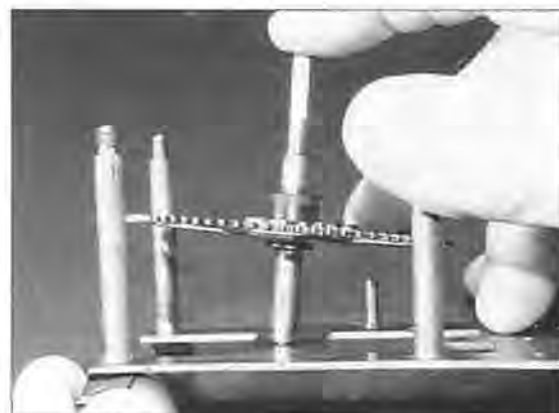
Figure 2. Tip the great wheel. This indicates condition of pivot and plate hole. This one is nominally good.
