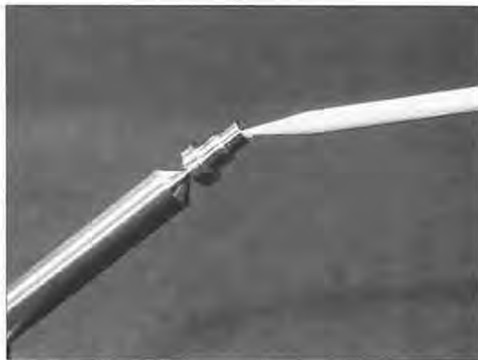
Figure 4. What you cannot see is a deep conical cup of about 60 degrees angle in the end.
