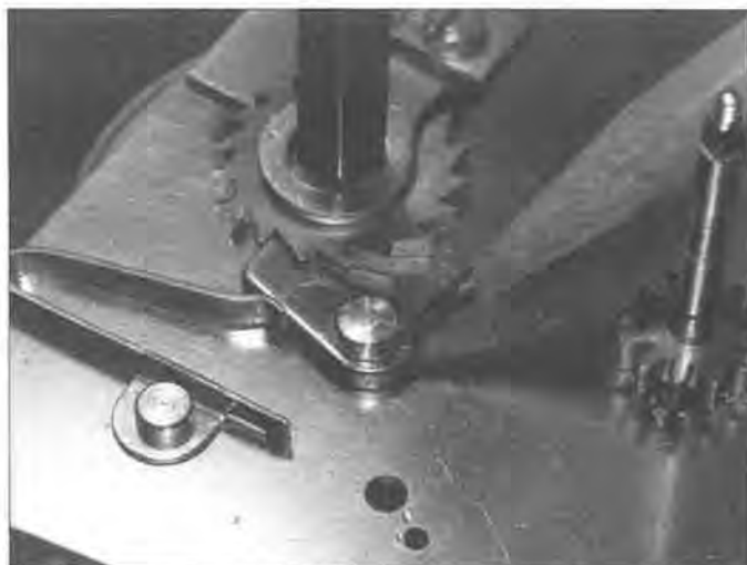
Figure 12. The large rivet is the job at hand. The small one is original to this AWI student practice movement.
