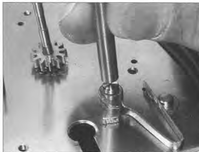
Figure 5. Use the raw material stock as a handle to assemble the pieces. Hold pressure downward and break away the handle.
