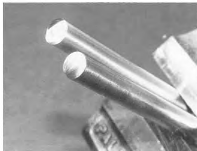
Figure 9. A bronze conical punch and a steel flat-faced punch did the job with a single stroke each.
