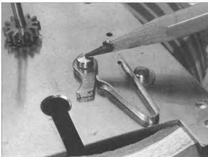
Figure 6. Breaking away the handle leaves a small bur on the rivet head. This head will be supported by a heavy bench block.
