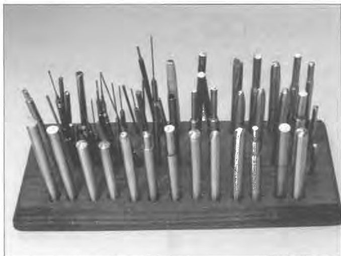
Figure 10. Clock staking punches: Most are over a half-century old. All are shop built of bronze and steel. Small pieces are broaches, pivot gauges, oilers, etc. All are active working tools.
