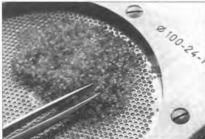
Jewels on Iron Plates for Grinding and Polishing
