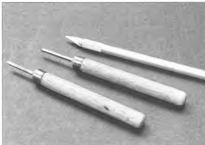
Figure 11. Lathe tools used in this article. Modified hobby knife ground as a cut off tool. Wood handles \frac{1}{2} inch diameter, 4 inches long. Tool bits are \frac{3}{32} inch square spring steel stock about 1\frac{1}{4} inch long.
