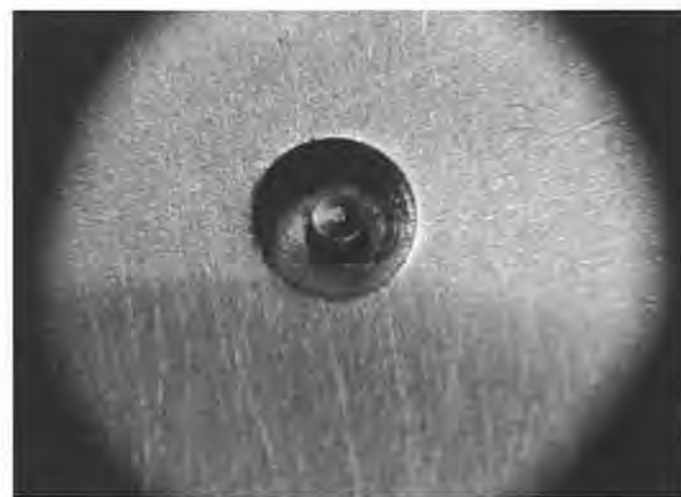
Figure 10. This original plate hole was opened, and then swage-closed and rebroached. It was photographed through a 15x eye loupe. Use discretion with this technique. Pivot diameter is \frac{3}{4} mm.
