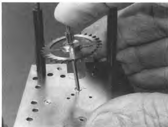
Figure 8. Overzealous broaching can end up like this. In some cases the hole can be swage-closed and rebroached. Use extreme discretion.
