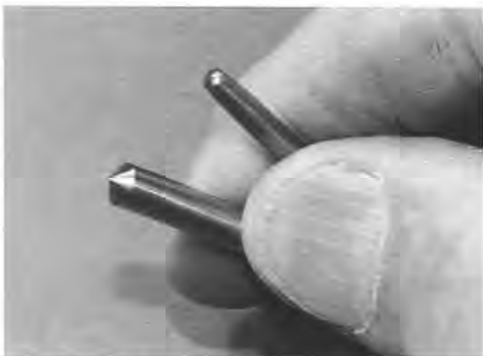
Figure 11. Bullet and swage used in this article. Bullets in Figure 1 are from about 0.118 to 0.126 inch diameter in increments of about 0.001 inch.
