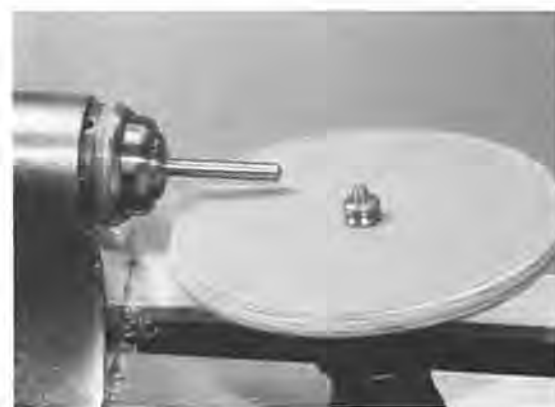
Figure 2. Bullets are made from short lengths of steel rod, of a precision size, cylindrical in the mid-section, and tapered to each end. I grind them to size as illustrated.
