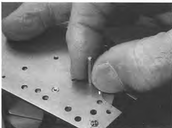
Figure 3. A bullet is either pressed or driven through a hole to form a precision diameter and internal finish.
