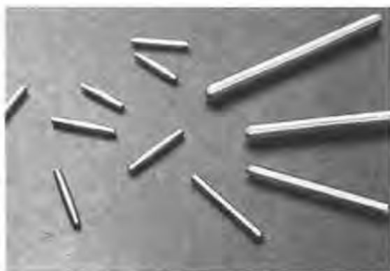
Figure 1. Shop-built staking tools: a ball punch, two swages, and a half-dozen bullets. These are tools for working brass.
