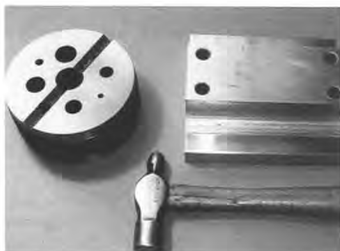
Figure 12. The tools used are a number 129 bench block by the L.S. Starrett Co., a piece of industrial scrap, and a Stanley #291B 2-ounce steel hammer.
