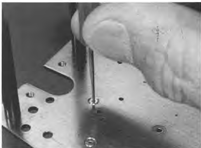
Figure 7. I broach the holes from both sides of the plate. That gives the hole a slight hourglass shape.
