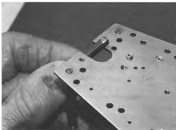
Figure 4. This swage has an included angle of about 130 degrees. It can reduce the hole size in our plate. The hole near the loose bushing is oversize.
