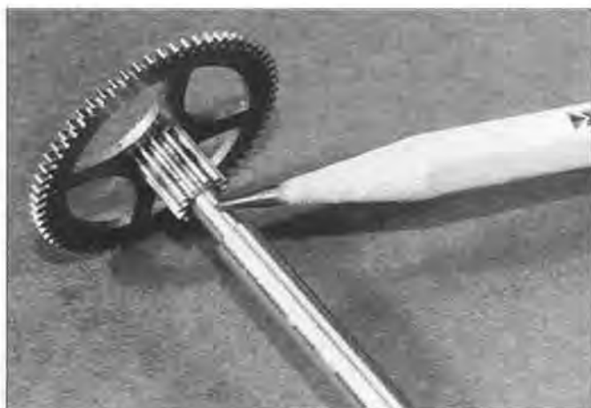
Figure 17. A larger arbor needs another tool. Do not anneal into the pinion.
