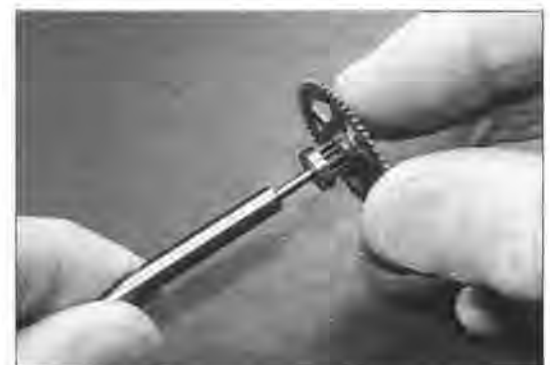
Figure 14. Annealing tool has a deep hole that the arbor will just slip in. The tool is a steel rod.
