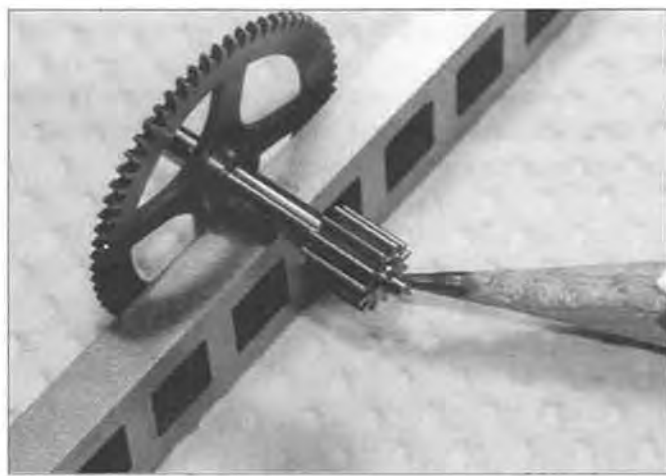
Figure 22. This is one of the most complex examples to anneal. Use a larger tool with a flat end. Do not anneal into the pinion's functional region.
