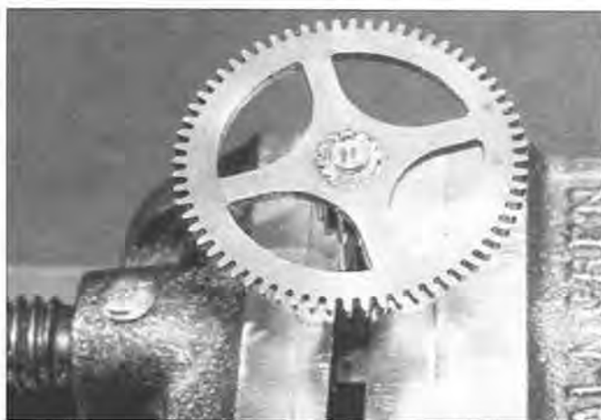
Figure 18. This one is unique. The wheel may need to be removed. A larger annealing tool with a flat end would be the choice.
