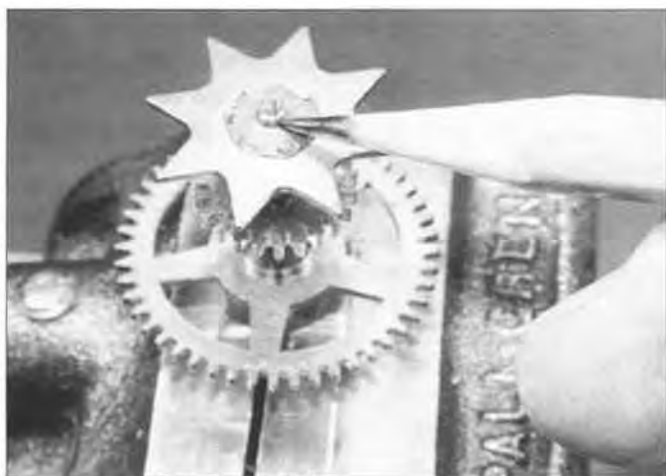
Figure 19. The star wheel must be removed, then the annealing tool is used.
