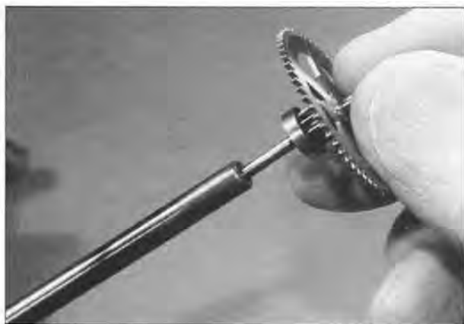
Figure 15. The tool is heated just beyond blue. Insert the arbor for a few seconds.
