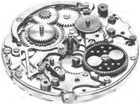
fig. 9-66 Perpetual calendar mechanism with 48-month cam in a Stangpaah watch.
