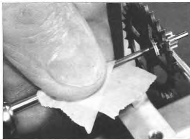
Figure 53. The tape coupling technique is my choice, where feasible. I'll use it for this job.
