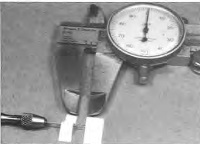
Figure 59. Tape the second bit and check depth. We read 0.201" which is 6-7 diameters deep. Depth is important to a good job.
