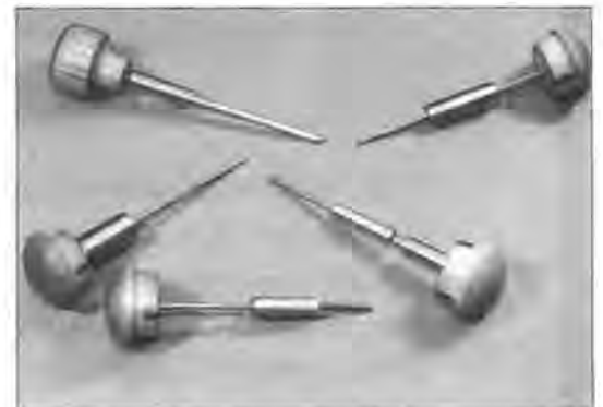
Figure 50. Examples of Huck's Magic Center Finder, a great time saver. I suggest you construct several sizes.
