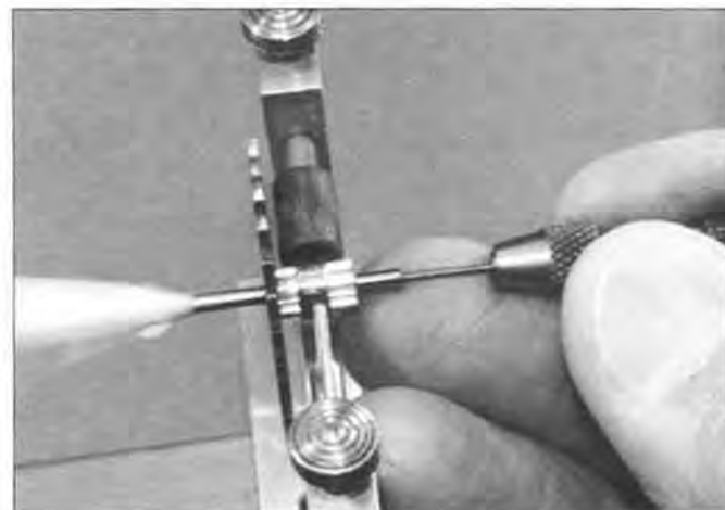
Figure 56. Pre-drilling: This bit is the exact size of the finished pivot. Diameter is about \frac{3}{4} mm and one-diameter deep.
