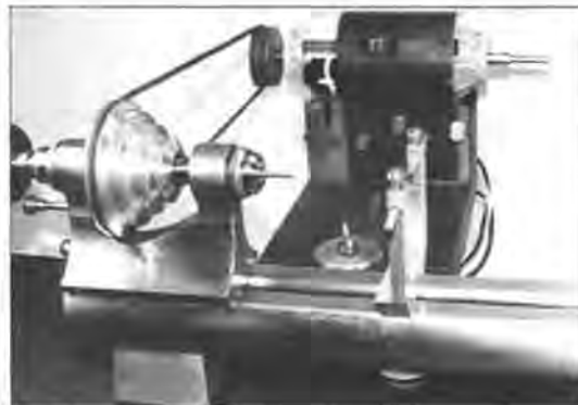
Figure 49. Lathe requirements are simple: a steady rest, a collet and brass rod, and not excessive slack in the bearings.
