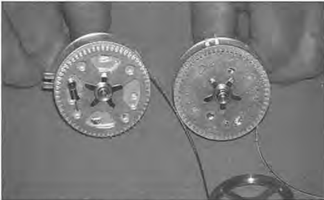
Figure 4. UW66 series time drum left and strike drum on right. Note click spring protruding from bottom semicircular cutout on both gears. Spring must be pushed toward center to release click.
