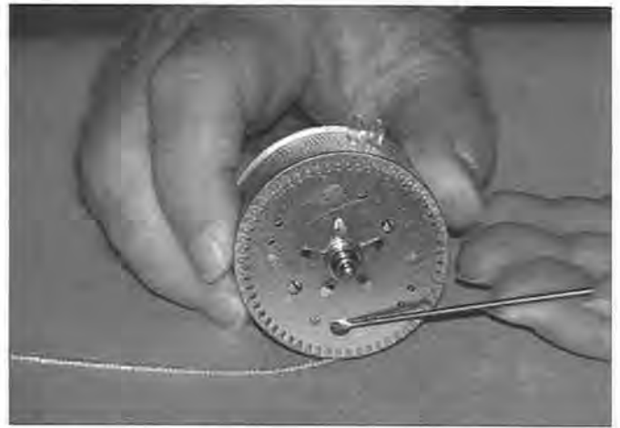
Figure 5: Pushing click spring toward center.
