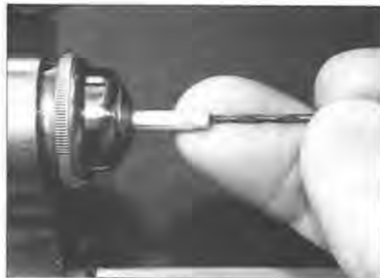
Figure 85. A finger held bit drills a 1/8 inch wood dowel to make a pivot polishing bed.
