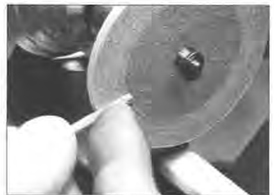
Figure 86. Grind away the dowel to make a "half-open" pivot bed.
