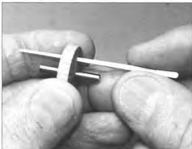
Figure 88. A brass rod with two cup centers, wood disc and toothpick—a perfect driver for pivot work.
