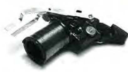
Original Accutron 219 Cell Coil #715
