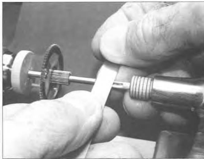
Figure 93. A flexible steel burnisher is used on this pivot.
