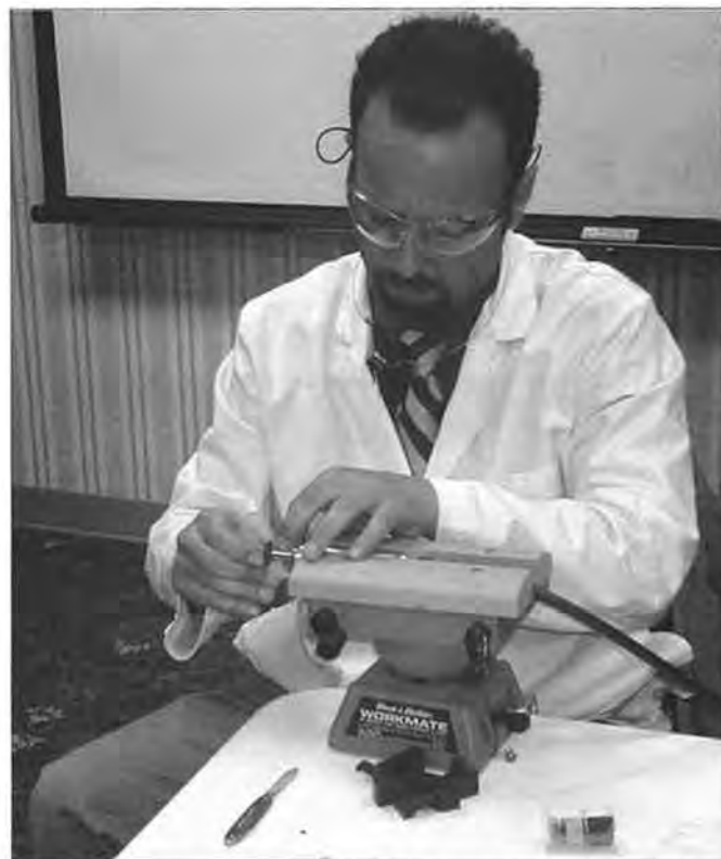
Manuel Yazijian making a specialized collet removing tool.
