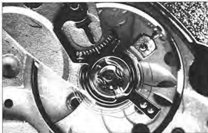
Centering the hairspring and collet without the upper jewel in place.
