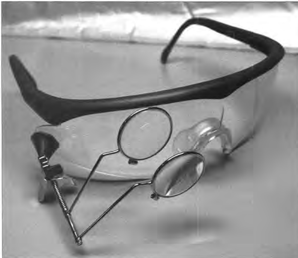
A pair of Bobster® Eyewear safety/shooting glasses with a Bausch & Lomb 3X-5X eyeglass loupe attached. Note the crack just above the nose bridge.
