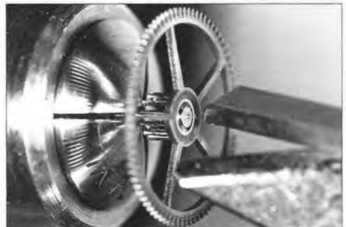
Figure 29. The pivot was removed and a perfect center was cut in the shoulder.
