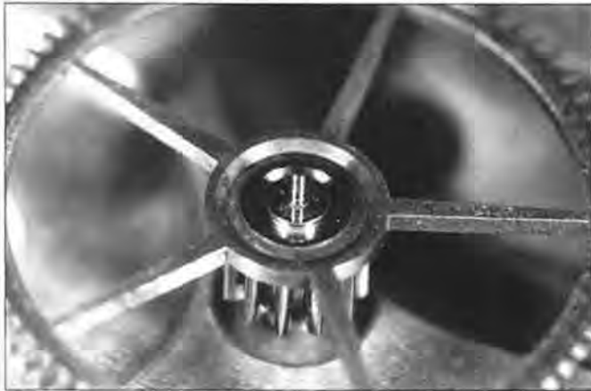
Figure 26. The center wheel pivot had been turned down in the past.
