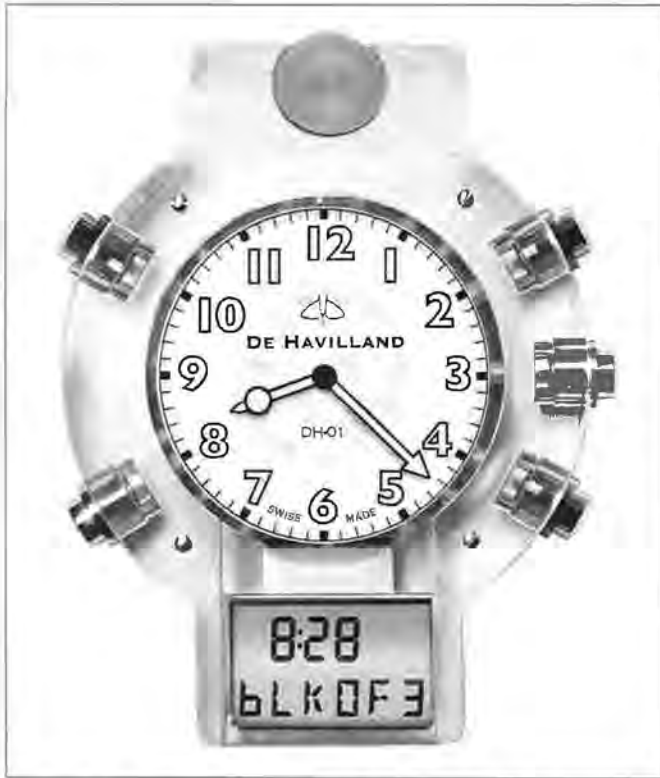
Figure 3. Watch demonstrator: the upper knurl simulates the functioning of the bezel. The push buttons are not linked mechanically to the movement. The LCD and movement are linked.
