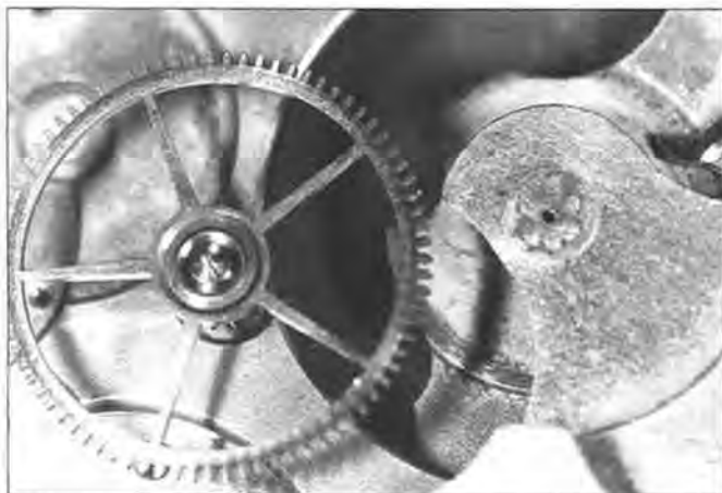
Figure 27. The center wheel pivot hole had been punched closed as evidenced by the marks surrounding the pivot hole.
