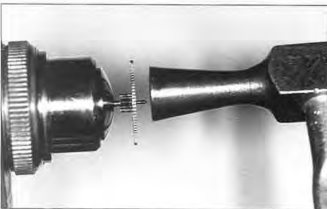
Figure 37. The new pivot was gently tapped home.
