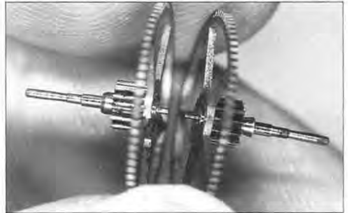
Figure 28. The turned down pivot compared to an original size pivot. Even the original pivot seems quite small for a center wheel.
