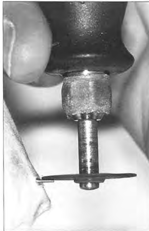
Figure 33. A piece of blued steel was ground to fit the hole. The lathe was shrouded to protect it from grinding debris.
