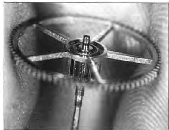
Figure 39. The substantially larger finished pivot
