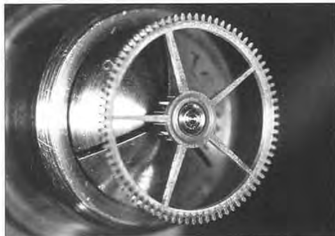
Figure 32. The hole was drilled larger than the final pivot diameter.
