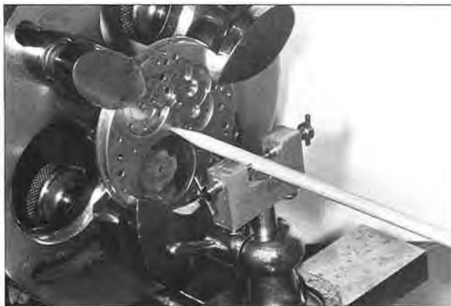
Figure 41. The center wheel hole was centered using a wobble stick.
