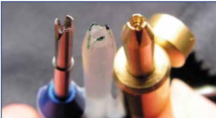
Figure 5: Comparison – Original tool, my acrylic version, my brass version
