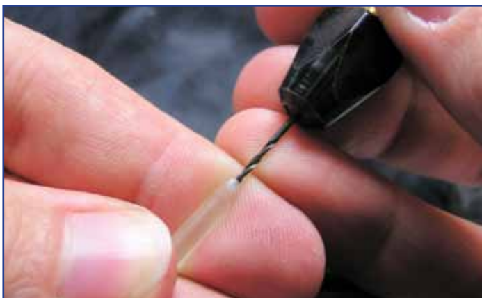
Figure 2: Step 3 – Drill center hole by hand
