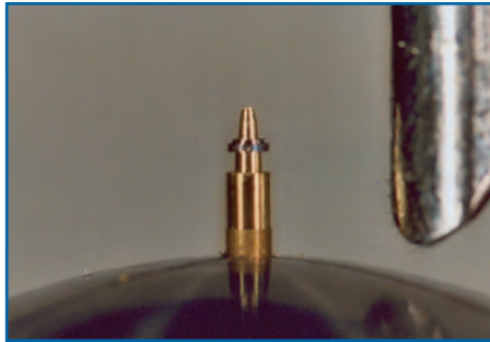
Figure 12. A mandrel was turned out of brass to support the tiny bushing and the bushing's height was reduced approximately one half.
