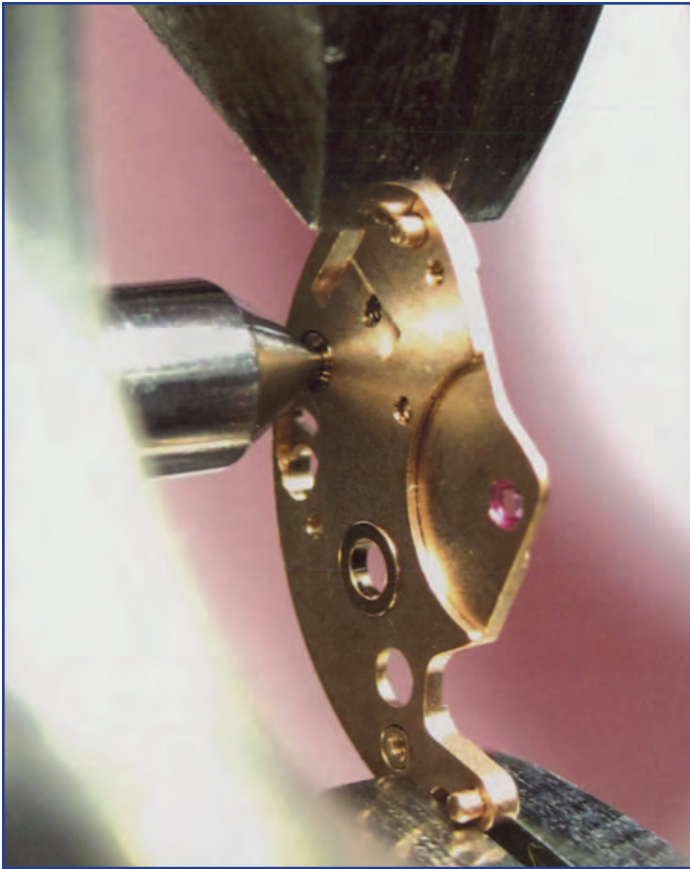
Figure 4- The face plate pump center was used to initially locate the post on center.
