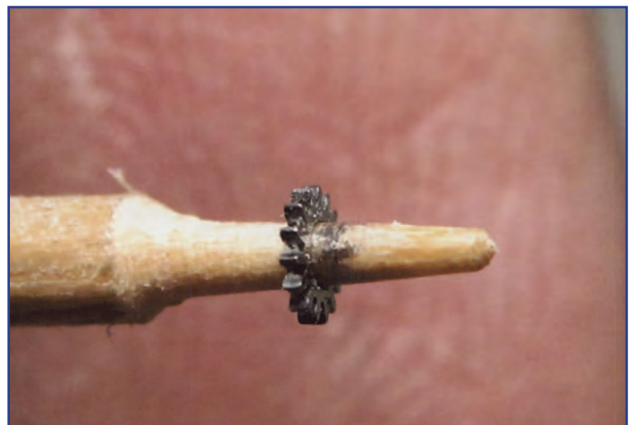
Figure 12- The inside diameter of the intermediate wheel was polished with diamantine.
