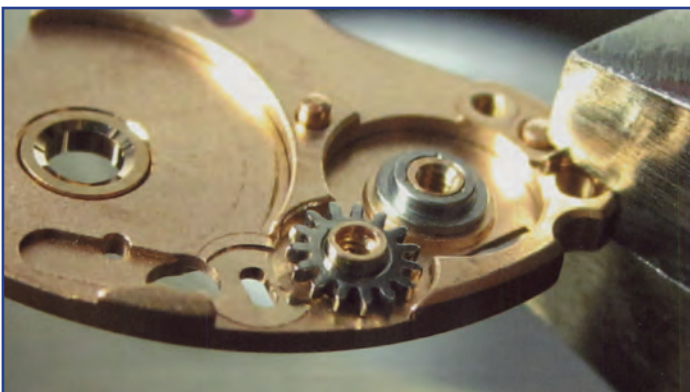
Figure 13- The wheel and post were returned to their original positions.
